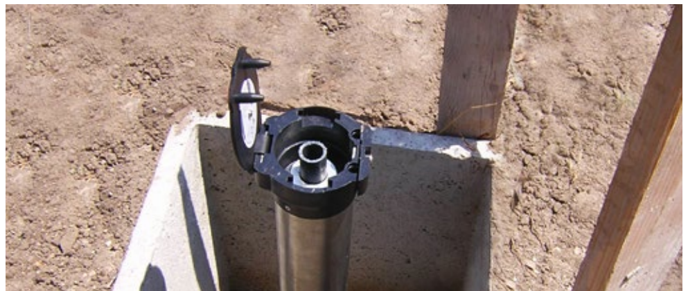
Tell - tale measuring head without survey pin
